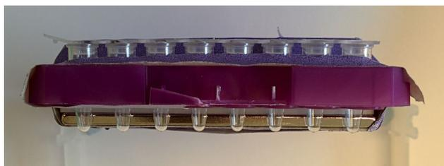
**Important:** as the magnet needs to remain firmly in contact with the edge of the strip tubes at all times, use a second PCR strip and/or tape on the side of the strip to hold the magnet in place.
